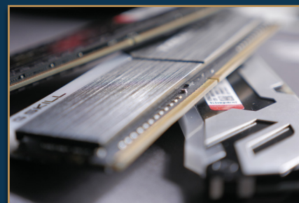
Memory heatsinks come in all sorts of shapes and styles but often they're not doing all that much for cooling
