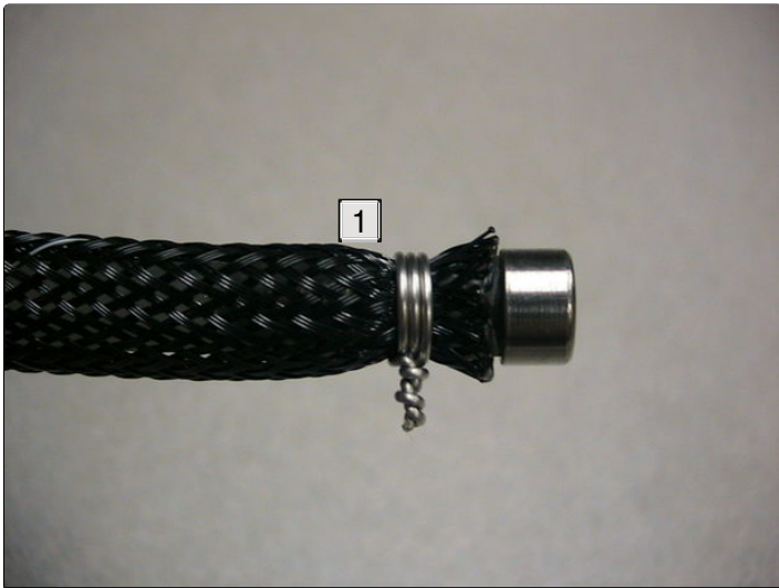
1. wrap ends with safety wire and tighten
