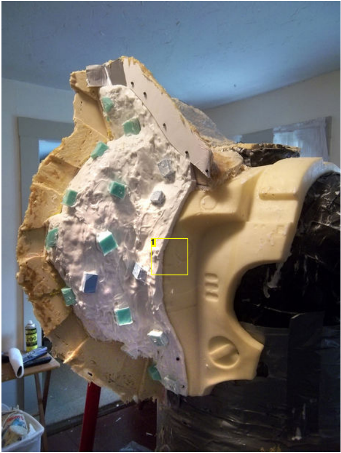
Image Notes 1. This shot shows the parting lines for the mold
