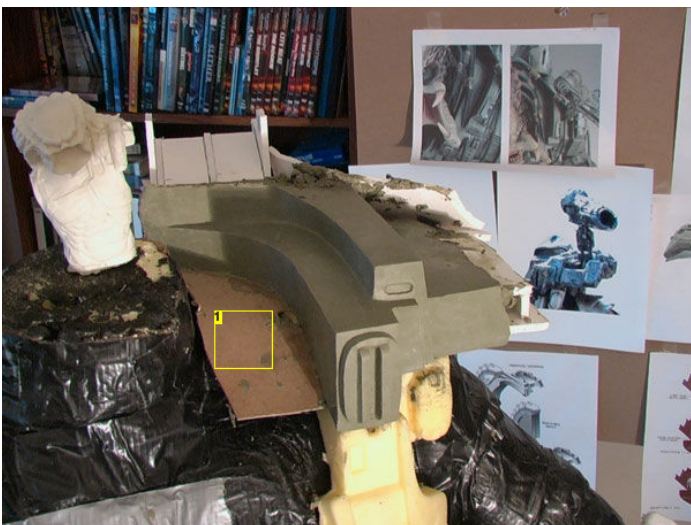
Image Notes 1. Foam core skeleton- this is cut roughly in the shape of the backpack to save clay 2. Foam torso armor
