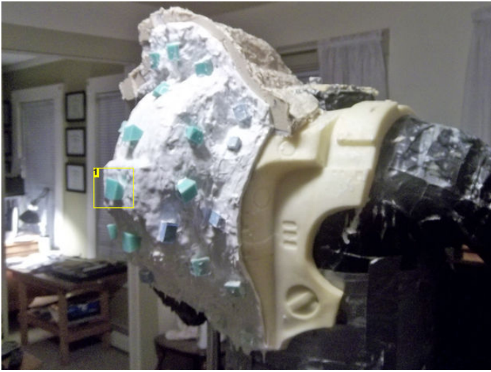
Image Notes 1. The little blocks of silicone material are keys for the reinforcing mold jacket
