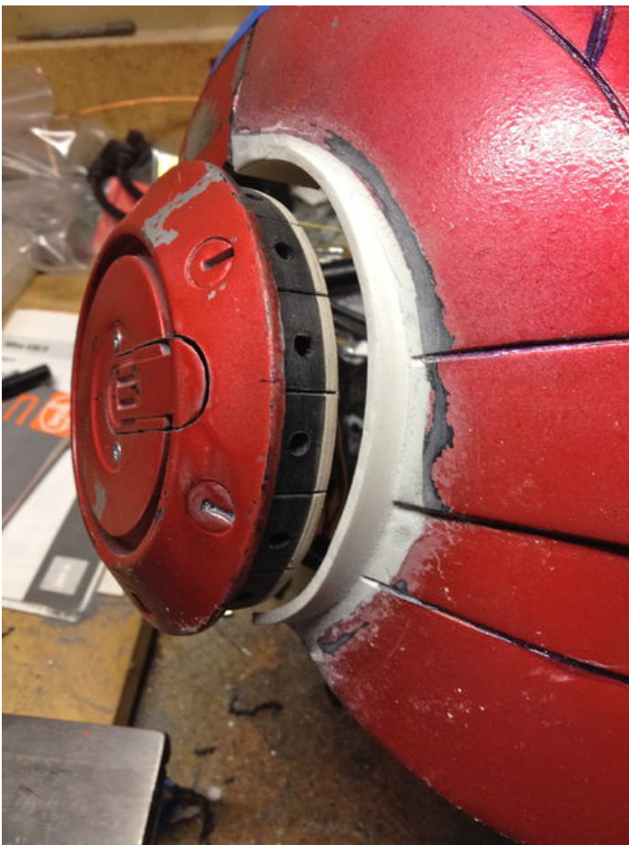
Image Notes 1. Pod cover rotation servo 2. Wiring for hip pod LEDs with 100 Ohm resistors
