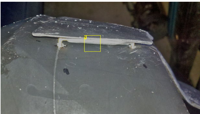
Image Notes 1. Brass rod and tube hinge epoxied to the underside of the flap
