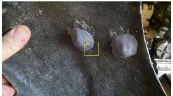
Image Notes 1. ProPoxy 20 epoxy putty is formed around the hinge rods to hold the hinge in place
